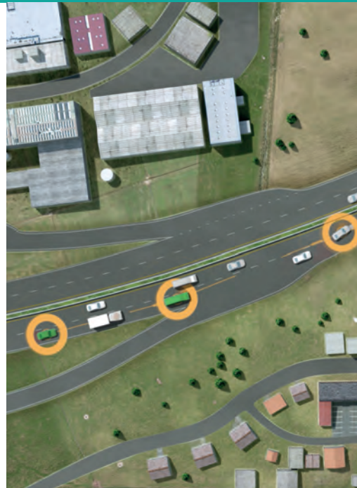
Right: Vehicles further along the road can inform following vehicles of the need to slow down in advance
