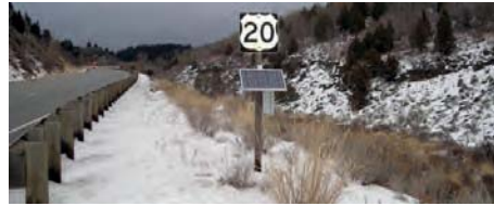
Left: Roadside weather stations communicate traveling conditions to traffic managers
