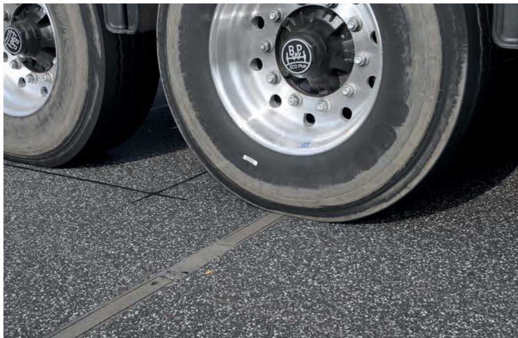
Right: WIM-DSP 32/TMCS-U is the world's first and only OIML R134-certified low- and high-speed WIM system
