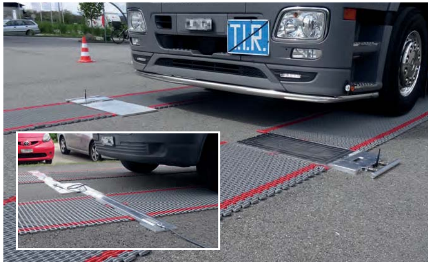
Left: Type WL 108, for certified static weighing
