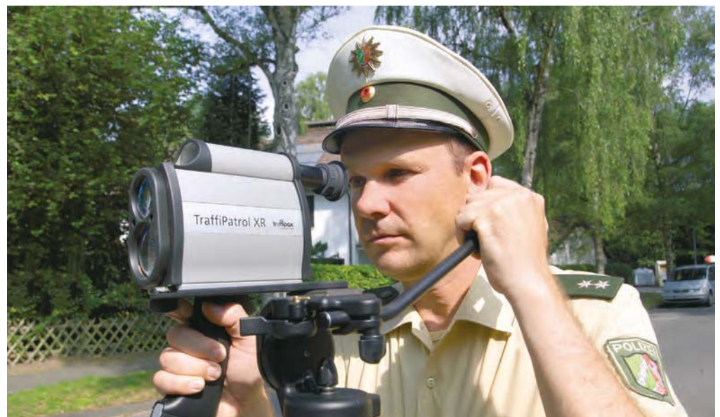
Below left and right: Handheld laser cameras are typically pointed at license plates to get a speed reading, however pointing at other points on a car can defeat jammers
