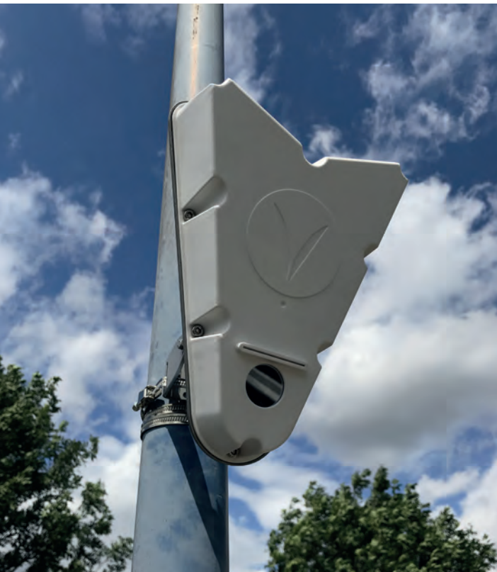
Below: Intelligent sensors deployed in Milton Keynes, UK, enable signals to react to traffic congestion
