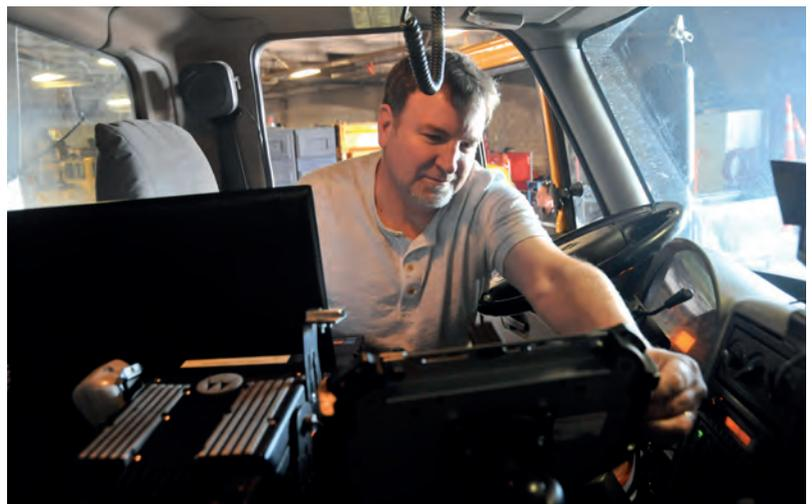
Right: Installing an OBU into a snowplow cab. It is planned that a total of 400 vehicles will be involved in the Wyoming pilot
