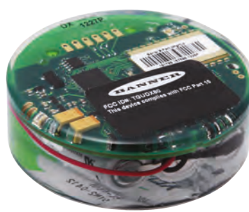
Left: Magnetometers measure changes in the ambient magnetic field
