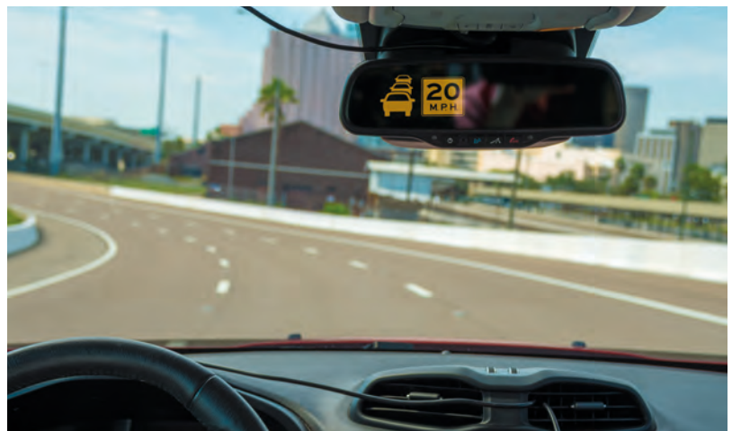
Right: An in-vehicle speed limit warning, displayed on a rearview mirror, that could be used in post-pilot operations
