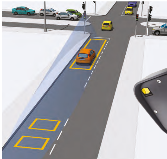
Left: AGD Systems' 318 pole-mounted radar replaces traditional loops
