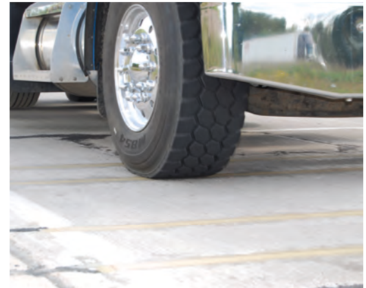
Left: The LS-WIM axle scale is suitable for weight enforcement Below: The strain-gauge strip sensor handles 80mph speeds
