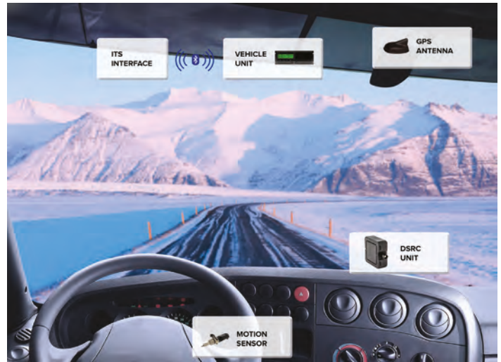
Above: DSRC for usage in digital tachographs Left: With high traffic volumes, electronic toll collecting has a role to play
