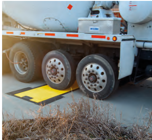
Left: The LS-WIM axle scale is suitable for weight enforcement Below: The strain-gauge strip sensor handles 80mph speeds
