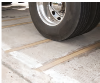
Above: Strip sensors are grouted into 3in (75mm) channels
